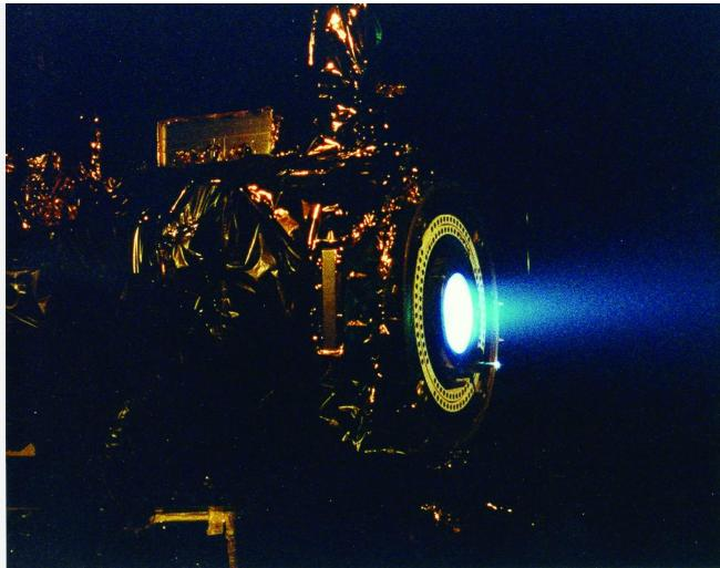
*Ion drives have low thrust but high efficiency. They have already been used on several space missions, including NASA's Deep Space 1spacecraft and Japan's Hayabusa asteroid sampling probe.*
