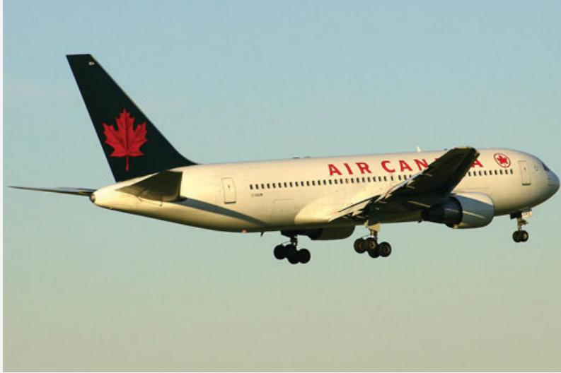
*The Gimli Glider is the Boeing 767 that ran out of fuel and glided to safety at Gimli Airport. The aircraft ran out of fuel because of confusion over the units used to express the amount of fuel.*
